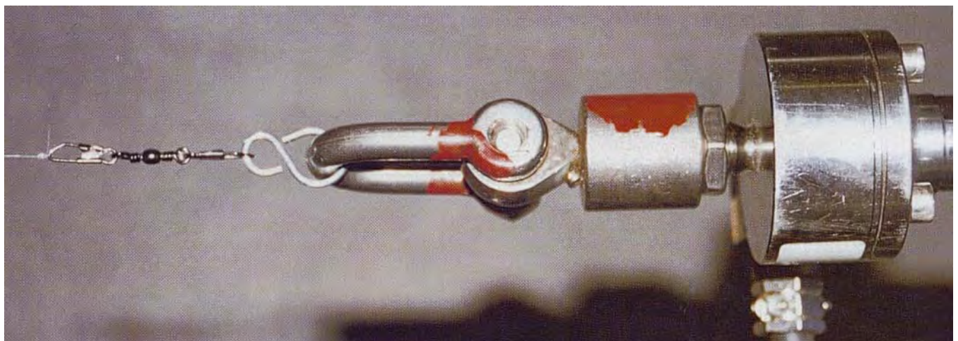
Above is the climatic chamber in which the lines were stored Below is the tensile stress machine head that was used to test the lines
